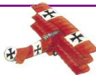
The Fokker Dr. 1 triplane was the favourite plane of German First World War ace Baron Manfred von Richthofen, known as the "Red Baron". It had a machine gun that could fire forwards without hitting the aircraft's own propeller.
