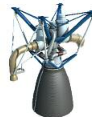
In a rocket engine, two different fuels mix and react together inside a combustion chamber. The hot gases created rush out of a nozzle (below) at high speed. These push the engine in the opposite direction.
